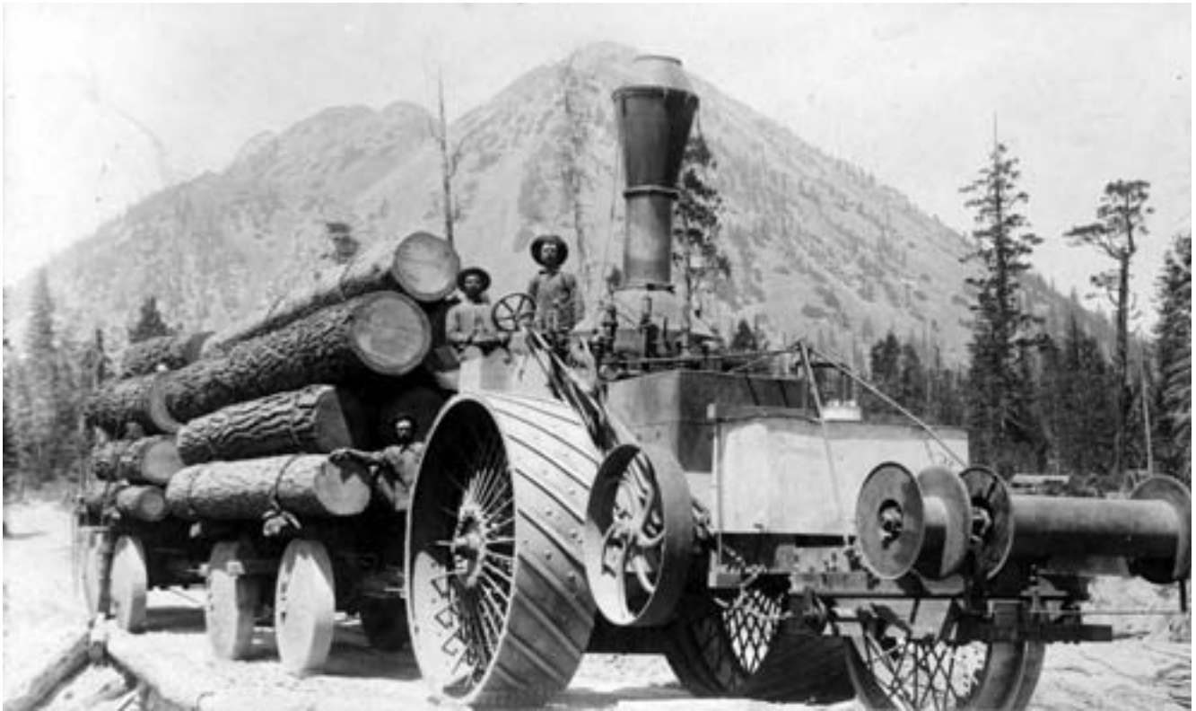
This steam tractor is rigged not only for skidding but also to serve as a donkey for providing power for various tasks at the logging site. Photographer: Andrews, circa 1888.
